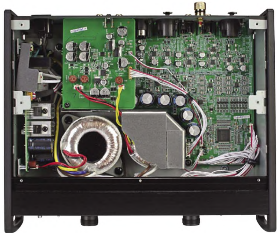
Inside, the distinctive round shape of a toroidal mains transformer, part of a linear power supply. At lower right is the square outline of a microprocessor.
