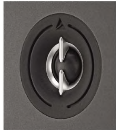
The EFS silk-dome tweeter is partially horn loaded and powered by a neodymium motor coupled to a cooling system for improved power handling.
