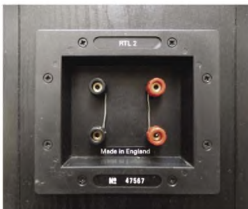
The RTL2 can be bi-wired – or indeed bi-amped. Some users have claimed excellent results from the latter. Note the dodgy stiff-wire links. 'Stressed' RTL2s can show evidence of melting, due to the overheating of crossover components on the other side of the terminal panel.
