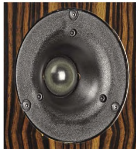
The 1in (25mm) silk dome tweeter sits in a shallow horn to improve sensitivity.
