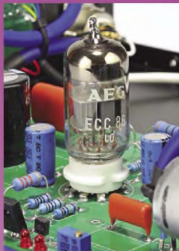
A NOS (new old stock) AEG ECC 88 double triode valve that acts as buffer between source and power amplifier.
