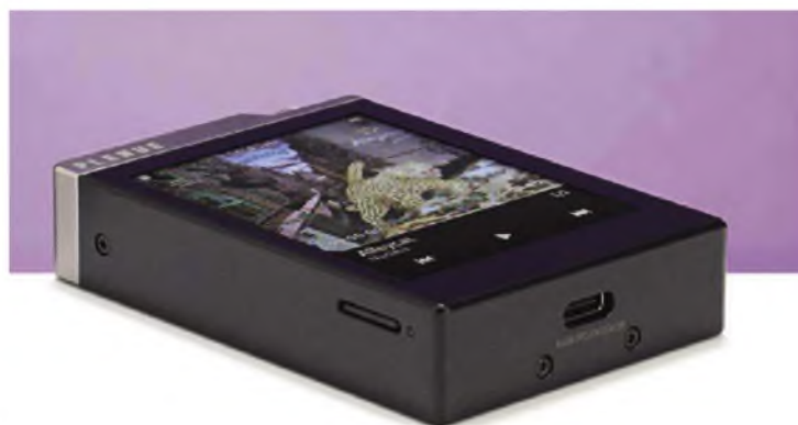
At left a single microSD card slot able to read cards up to 128GB. On the base is a USB C socket (that accepts a plug either way around) for charging and connection to a computer, in order to load the internal memory.
