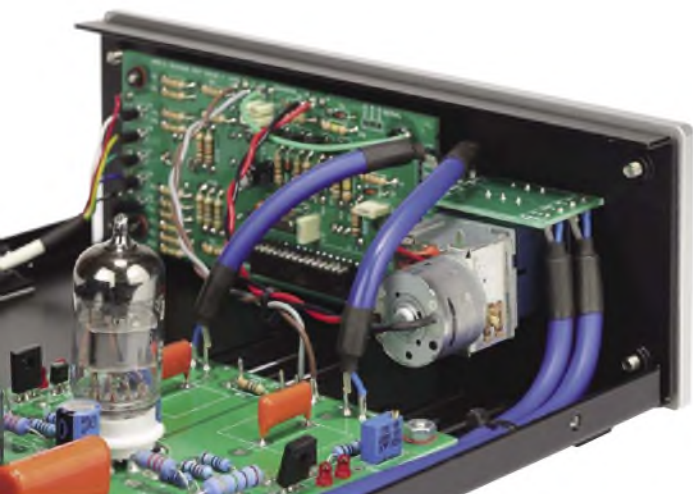
The remote control and rotary actuator board at left, and an Alps Blue motorised potentiometer (volume control) at right, driven manually or by the remote board.
