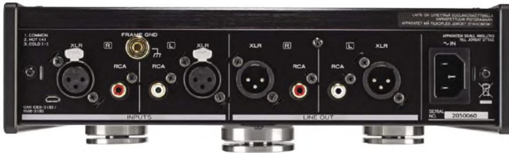
Big gold earth terminal sits between XLR and phono inputs. At right are the outputs, the XLR sockets giving double (+6dB) more than the phono sockets.
