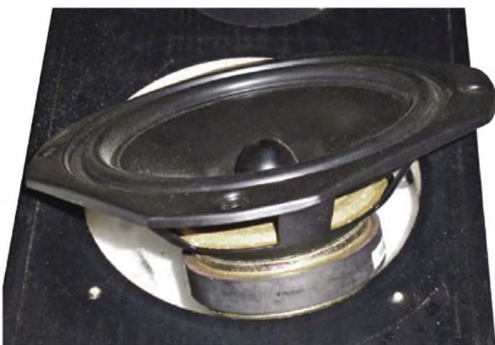
A sideways view of the RTL2's ELAC-made woofer – you can also see into the cabinet, which is lined with acoustic wadding. Unfortunately, no 'officially-compatible' replacement for this driver is available today.
