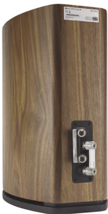
The rear view shows a curved cabinet to discourage internal standing waves, bi-wire terminals with mono wire links, and a small gap between base and cabinet. This provides clearance for a down-firing port, the narrow gap providing a measure of acoustic damping.
