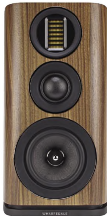
An unusual drive unit line up comprising folded ribbon Air Motion Transformer treble unit at top, fabric dome midrange at centre, and bass unit with central parasitic dome to cover lower midband at bottom.
