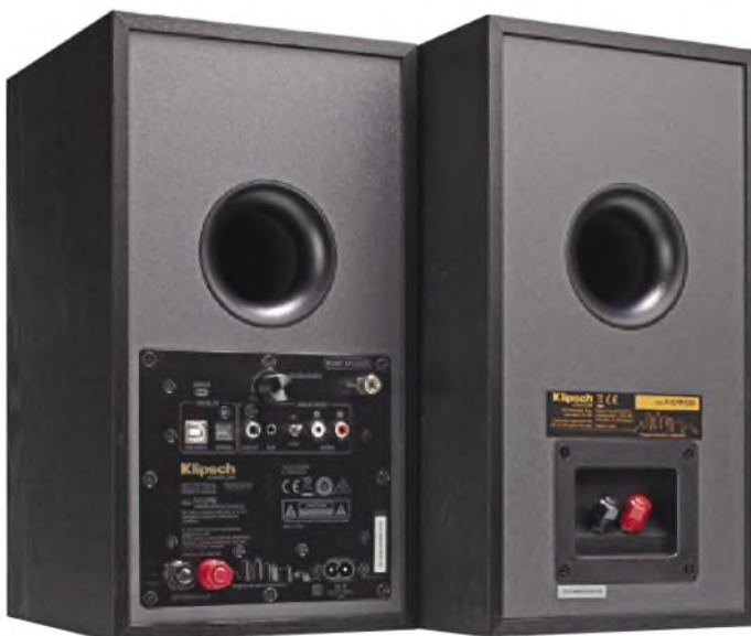
One loudspeaker (Right channel, seen at left from rear) carries 60 Watts per channel Class D amplifiers, a digital-to-analogue convertor, Bluetooth wireless and a phono stage for a turntable. A computer can be connected via USB B. The Left channel is an unpowered slave, connected by a slim cable.
