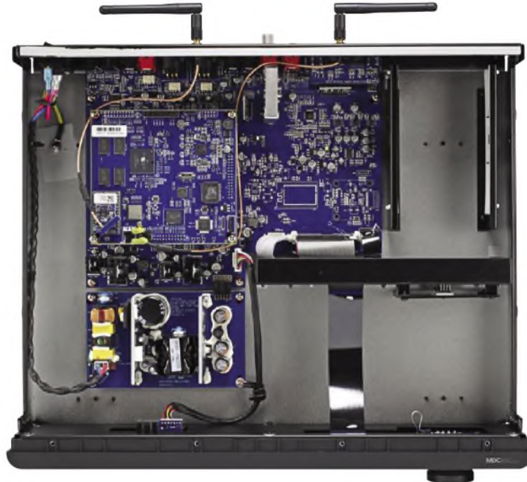
There are external wi-fi and Bluetooth aerials for efficient radio connection. Inside lie densely populated circuit boards full of huge chips, including the ESS DAC (near centre). Switch-mode power supply (screened) so no mains transformer visible.
