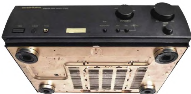
One of Ken Ishiwata's tweaks was to plate the PM66-SE Ki chassis with copper – claimed to improve performance by reducing magnetically induced eddy currents.
