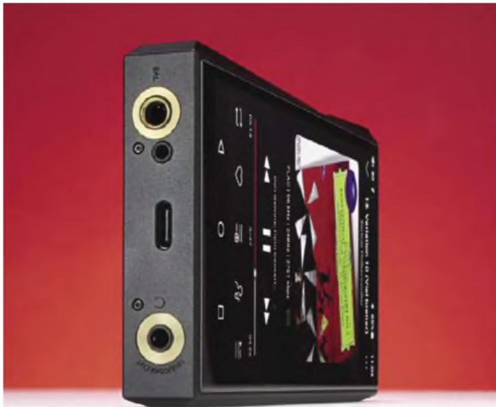
On the bottom face lie a conventional 3.5mm three-pole headphone jack that can be set to line output or deliver S/PDIF digital through an adaptor cable. Also, there's a USB C socket and 4.4mm four-pole balanced output (top) with 2.5mm (black) alongside.
