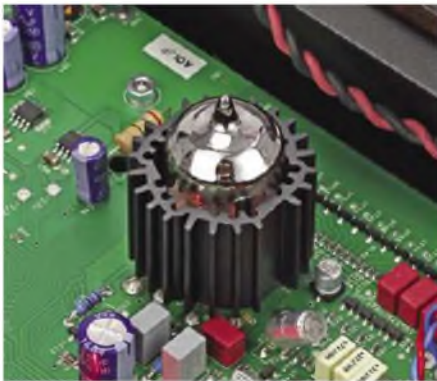
Clip on heatsinks help cool the valves, but they only run warm in any case.
