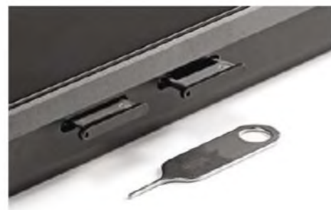
The microSD card carriers fit one way only and extraction is with the tool supplied.
