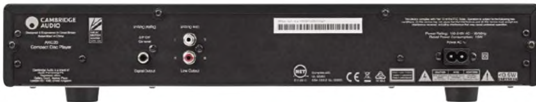
AX C35 CD player with electrical digital output at left, analogue outputs and 'calculator' mains input socket (right) – unlike the AX A35 amplifier that uses an IEC mains input.
