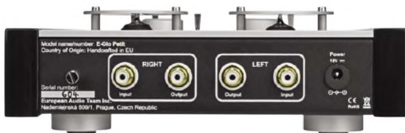
A simple rear panel carrying solid gold plated phono socket inputs and outputs. The unit is 'Handcrafted in EU, Czech Republic'.
