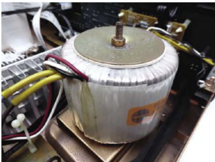
Ishiwata replaced the PM66-SE's conventional mains transformer with this expensive toroid – that likely accounted for a sizeable slice of the price difference.
