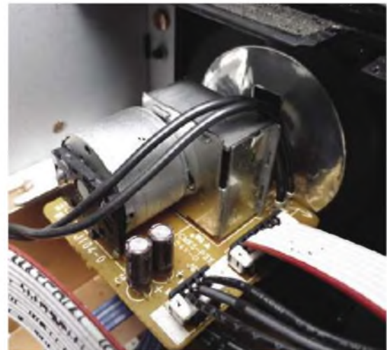
The volume control of the PM66-SE Ki (and the PM66-SE on which it's based) is motorised for armchair operation by remote control.
