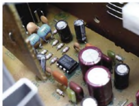
The PM66-SE Ki's moving-magnet phono stage was based on a NJM2068 dual op-amp, giving an introduction to the joys of vinyl.
