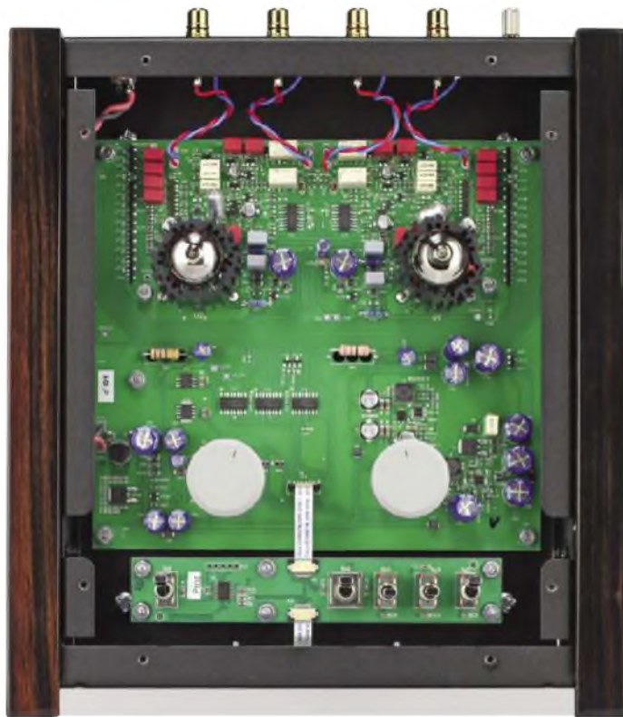
Neat circuit boards carrying soldered-on switches, rotary and lever style – hence top panel controls. The valves with finned heatsinks are at top.
