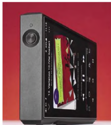
The top face carries a single on/off and wake-from-sleep button. Power up is quick at 15 seconds.
