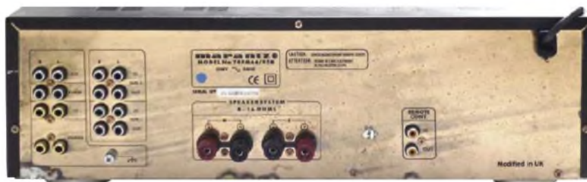
The PM66-SE Ki is resolutely an analogue-only design. It makes provision for two tape decks (with dubbing from one to the other), three play-only line-level sources (CD, tuner and auxiliary) and a turntable equipped with a MM cartridge.
