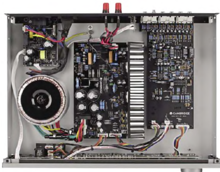
The AX A35 amplifier has a linear power supply with toroidal transformer (left) and vertical heat sink at centre. It is powerful enough to drive efficient loudspeakers.
