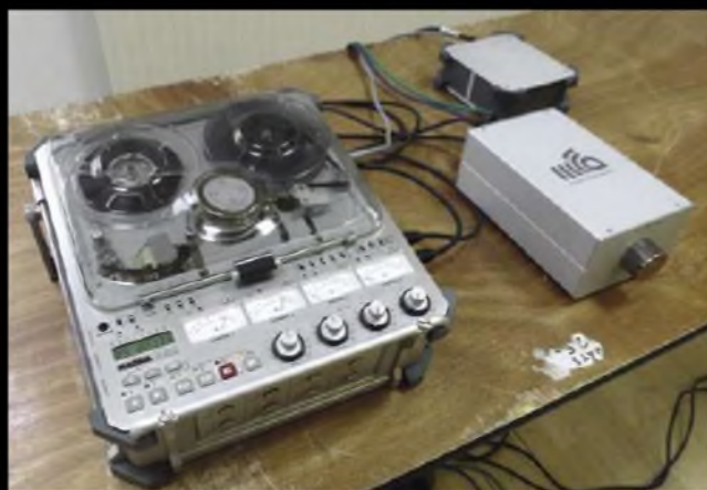
A professional Nagra 'D' four-channel 24-bit capable recorder that hitched quarter-inch tape running at a slowish speed to VCR-type helical scanning techniques. The guy from Music First Audio, who was using it as a demo source, told me he had one for sale for £4k...
