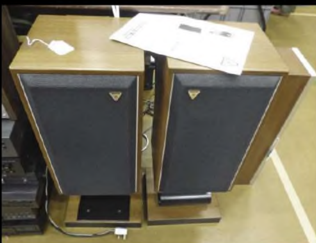
West Bromwich-based Griffin made speakers in the seventies. The 'Type 25', a ported and 'mirror-paired' design with a KEF B200 woofer and Coles tweeter driven via an 8-element crossover. The excellent condition of these ones reflected their £125 asking price.
