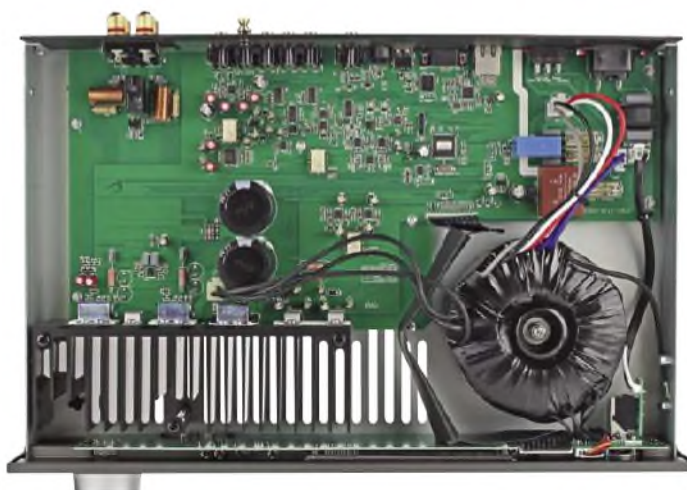
Interior of the Arcam SA10. The bottom left is dominated by the Class A/B power amplifier section and to the right is the enormous toroidal mains transformer feeding it. The top half houses the small-signal electronics (preamp, DAC and so on).
