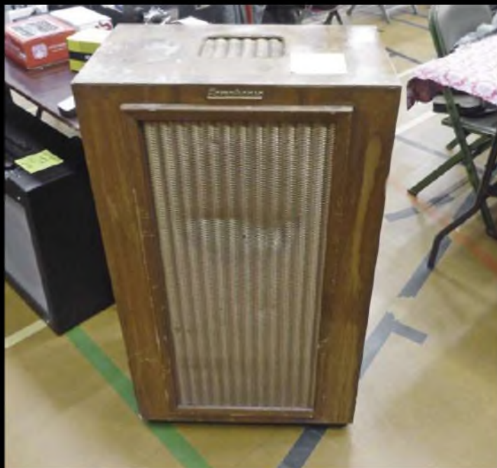
A tatty example of the imposing Pamphonic Reproducers Victor Senior loudspeaker from the mid-1950s. A 15in. woofer with enormous magnet and elliptically-coned tweeter. Yours for a tenner!
