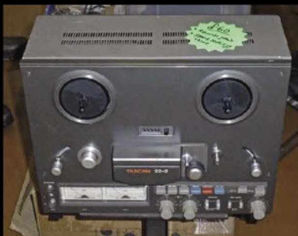
A compact 22-2 open-reel recorder from Tascam. Based on the TEAC X3, but with half-track format and higher tape speeds (15 as well as 7.5ips). Just 7in. spool capacity but an excellent introduction to the joys of analogue tape for a mere £60.
