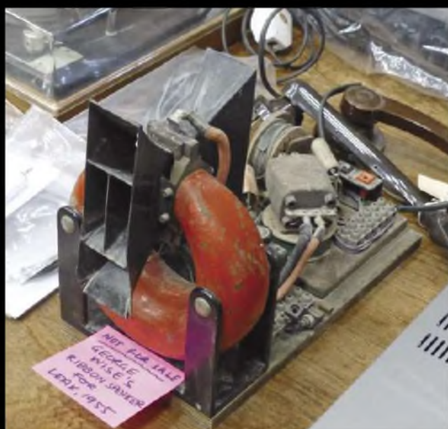
In the mid 1950s, Harold Leak commissioned fellow hi-fi pioneer George Wise to develop a ribbon tweeter. Pictured is the distinctive prototype of what Leak considered to be the "most faithful loudspeaker transducer until the advent of the electrostatic". Not for sale!
