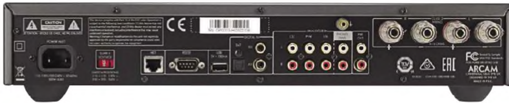
The rear panel carries an RJ45 ethernet socket, RS232 and USB at centre, for external control and software upgrade. At centre are S/PDIF digital inputs but no USB for computer connection. Then come analogue inputs and at right a single pair of loudspeaker output sockets for 4mm banana plugs, spades or bare wire.
