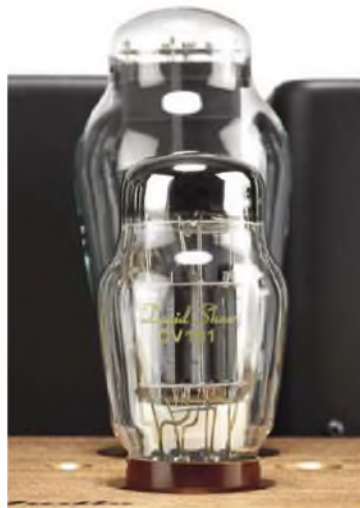
The 6SN7 (CV181) valves fitted both amplify and phase split to feed the 300Bs working in push-pull.
