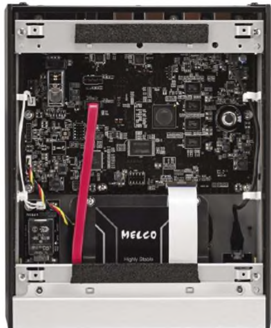
Internally, the N100 is a hugely complex network attached storage drive.
