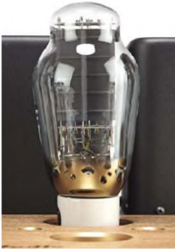
A 300B triode with its large, grey anode.
