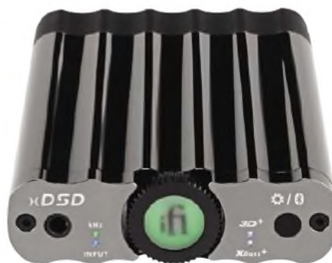
At centre lies an illuminated on/off button that changes colour with volume. Concentric is a knurled volume control. The tiny input LED (left, bottom) changes colour to indicate sample rate, or DSD.
