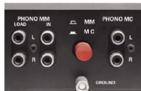
The Audiolab 8000A’s phono stage can be used with MM or MC cartridges. Both can be connected simultaneously - handy if you have two turntables.
