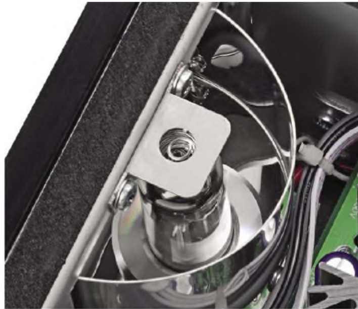
Behind the front window lies the 6Z4 rectifier valve; it is back-lit by an orange LED. Brightness is switch adjustable.
