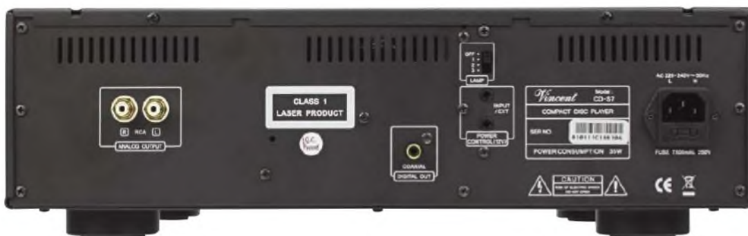
A very simple rear panel with little in the way of outputs, specifically no balanced XLRs. But there is an LED dimmer/off switch and S/PDIF digital output (electrical, via RCA phono socket).
