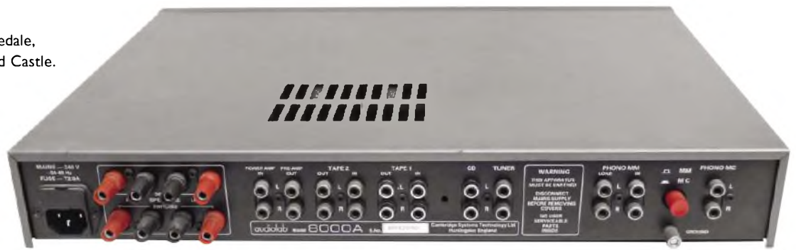
There are two sets of speaker outputs. One (‘direct’) is ‘always on’, while the other can be ‘muted’ with the front-panel’s ‘speakers’ switch.
