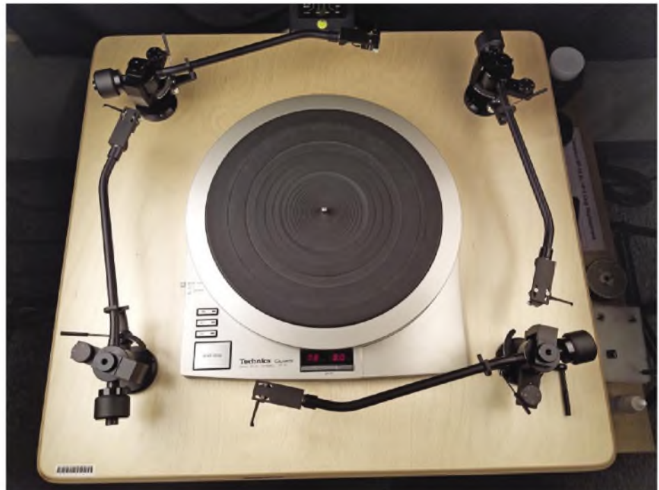
George Blood's Technics SP-15 turntable with four 12" Jelco arms attached. They carry Shure M44 cartridges with different stylus tip sizes to find a best match with uncatalogued 78s. See 'The Great 78 Project' box-out.
