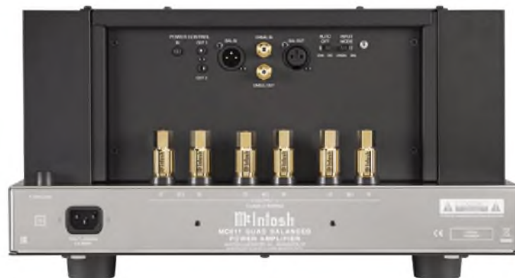
The rear carried 8 Ohm, 4 Ohm and 2 Ohm loudspeaker terminals in pairs, fed by dual-balanced internal circuits coupled through the output auto-transformer. Balanced and unbalanced inputs and outputs are provided.
