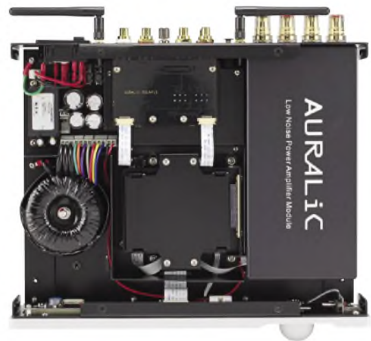
A toroidal transformer feeds the main power supply with shielding around the rest of the circuitry. Auralic have put great effort into the amplifier's internal lay-out.
