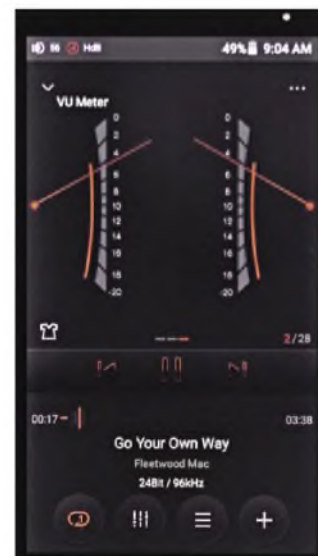
Entertaining VU meters show music level if selected, with PCM files only.
