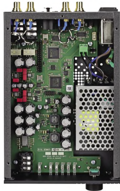
Note the switch-mode power supply module, in its screened case. The identifications have been ground off some devices. Identifiable are an XMOS microcontroller, Crystal digital interface and ESS DAC.
