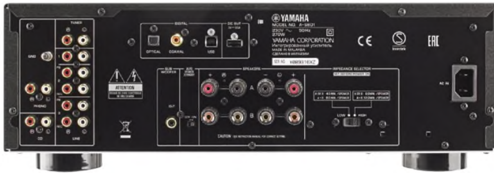
At rear are analogue inputs at left, including record in/out. At top lie the digital inputs and below two pairs of loudspeaker outputs able to accept 4mm banana plugs, spades or bare wire. A small slide switch to their right ensures matching to both pairs working simultaneously.
