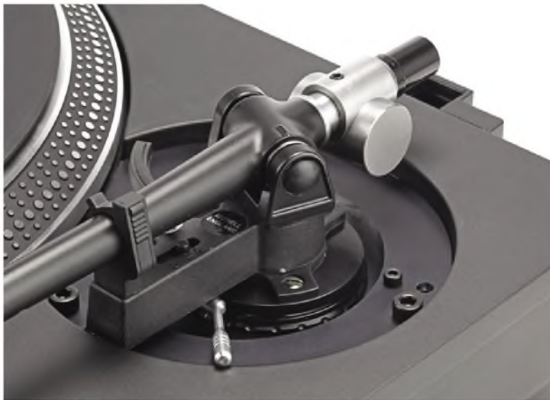
The Michell TecnoArm is based on a Rega RB202. Michell fit their own counterweight assembly, secured by a hex bolt and matching key. The lift/lower lever has little clearance beneath it, making use slightly awkward.
