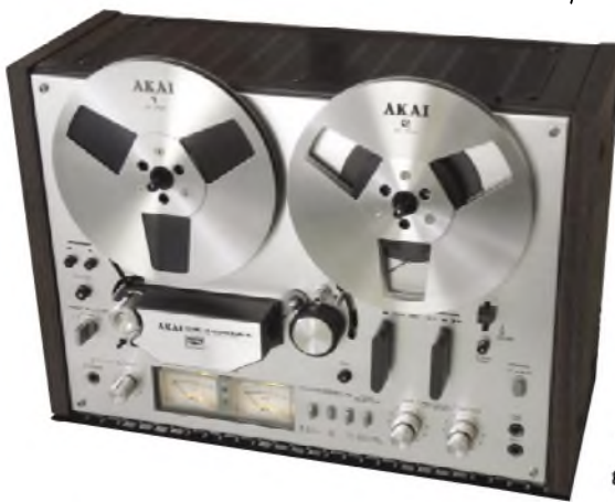
The Akai GX4000 (above) was very popular in its day; it used hard glass crystal (GX) heads that suffered little wear. Another popular open-reel recorder was the Sony TC-377 (below).
