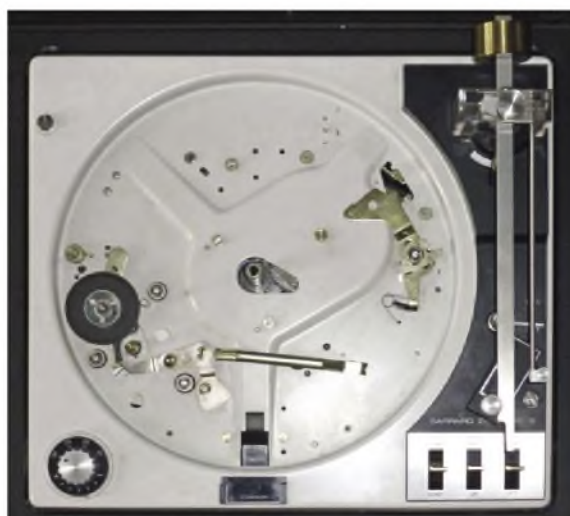
With the platter removed (a plastic disc is removed from the centre of the platter, to reveal a circlip), the motor pulley and idler are clearly visible. The linkages push the idler against the inner-surface of the platter when playing records, retracting it when the deck is off to avoid the possibility of 'flats' (and audible 'wow').
