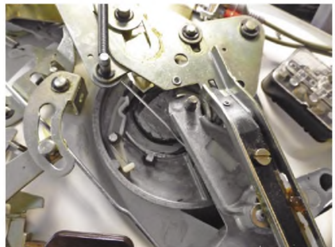
A diecast cam-wheel meshes with teeth at the base of the turntable bearing. It facilitates the Zero 100S's automatic operation – which is great for users who don't feel comfortable with manual cueing.
