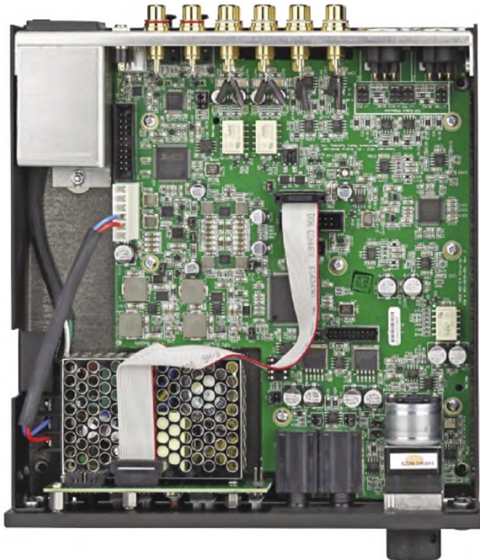
Inside the metal box at bottom-left is the switched-mode power supply, next to it are the headphone sockets and the motorised volume control that forms part of Benchmark's 'Hybrid Gain Control' system. The ESS9028 Sabre DAC sits at centre. The XMOS chip near the screened mains socket (top-left) forms part of the USB interface.
