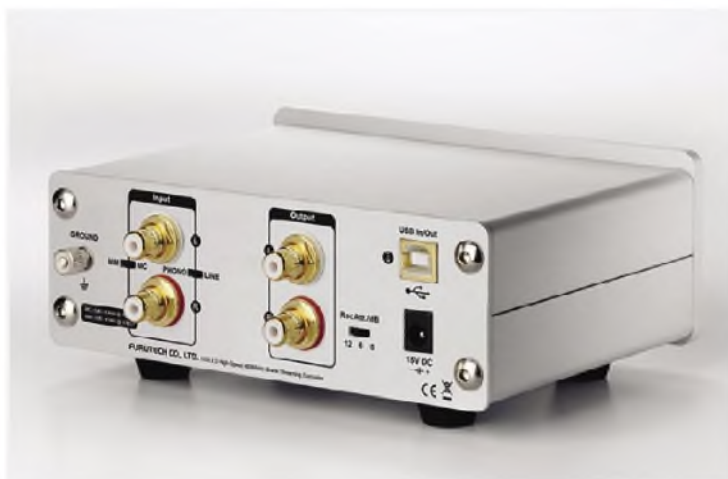
Furutech GT40 Alpha has on-board phono stage and digital output via USB. But it "doesn't want to talk to the Oppo BD105" says Jim Thorpe.
