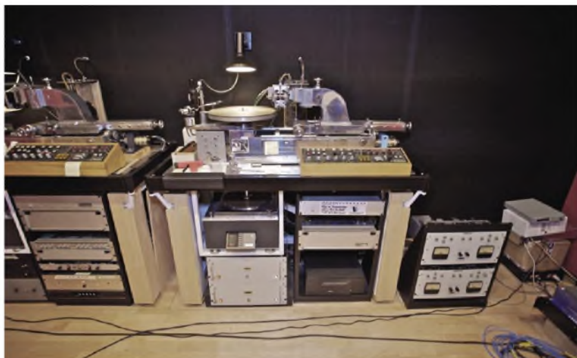
Doug Sax's The Mastering Lab. Included are Neumann lathes with Neumann cutting heads. All electronics have been designed and built by the Mastering Lab. itself.
