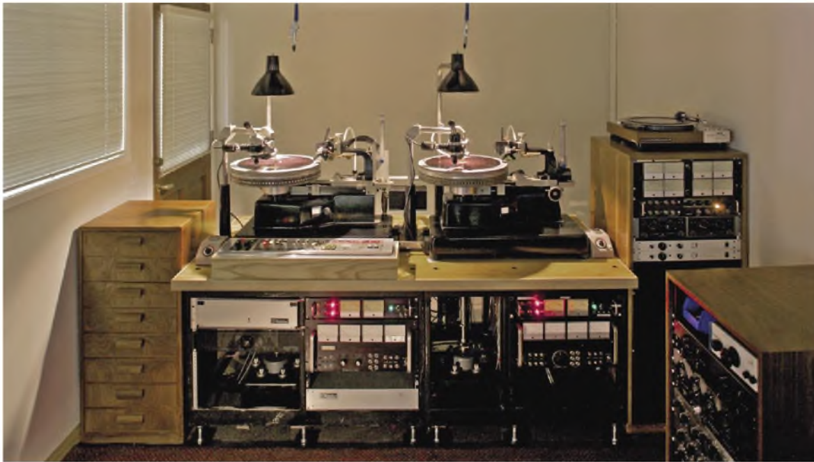
Grundman's facilities includes a valve-based Scully Lathe with Westrex Cutting Head and BGM electronics.
