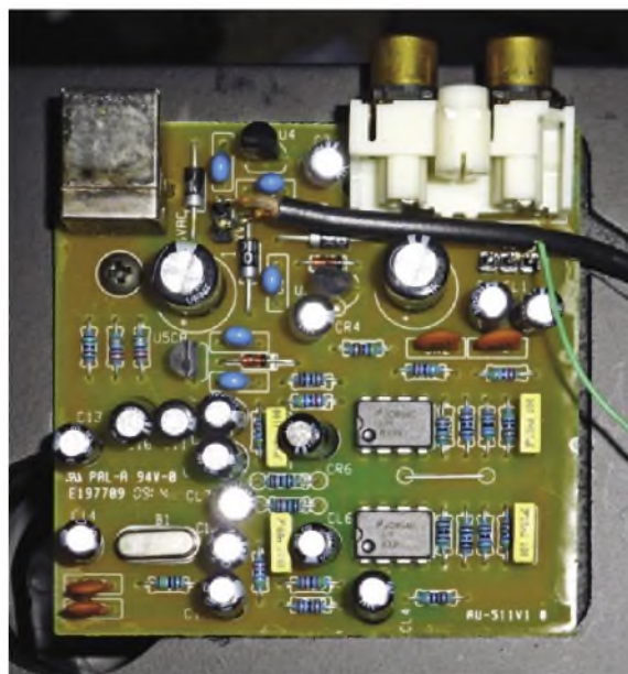
This circuit board, which lives in a metal box screwed into the base of its plinth, is the simple but effective phono stage and USB converter. The LM833N op-amps of the RIAA-equalised pre-amplifier, a crystal (associated with the digital converter and USB interface chip on the other side of the board) and power-supply components are all visible. Similar circuitry is used on Pro-ject decks to this day, although the firm will soon be updating the converter to a more worthwhile 24-bit resolution.
