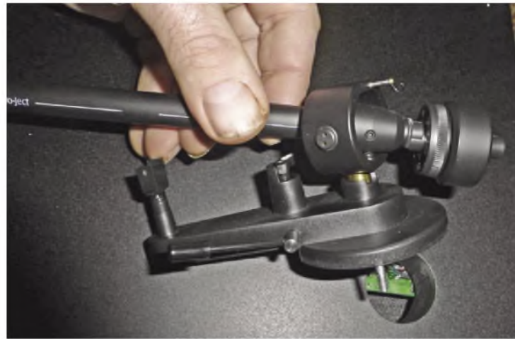
The simple but effective 'Pro-Ject 8.6' tonearm is secured to the Debut III via two bolts. Bearing 'play' is sometimes a problem – and the tonearm in the picture is being removed to sort that out!
