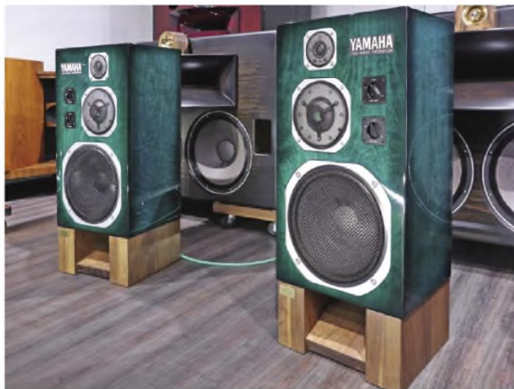
A lovely looking pair of restored and tweaked Yamaha NS-1000M loudspeakers from Japanese supplier Kenrick Sound ( http://kenricksound.com ). Note the big beryllium dome midrange units.
