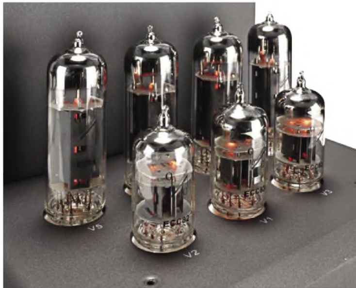
The valve complement, two pairs of EL84s operating in push-pull at rear, and ECC83 plus ECC82 double-triodes acting as preamp/phase splitters.
