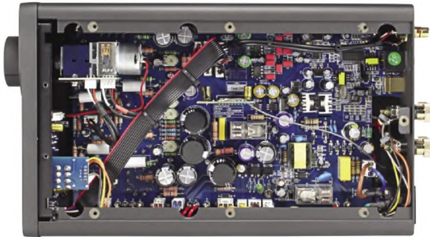
The busy internal construction of the VA-One. With most of the electronics on a single circuit board, volume production is eased - and costs reduced. I kept the VA-One running continuously for listening periods of 12 hours, with no ill-effect. Note the big Alps Blue motorised volume control at top left – a quality item.
