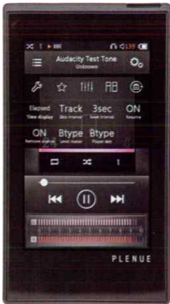
Red bargraph music level meters are a display option. Above them are touch screen transport controls that duplicate the side buttons.
