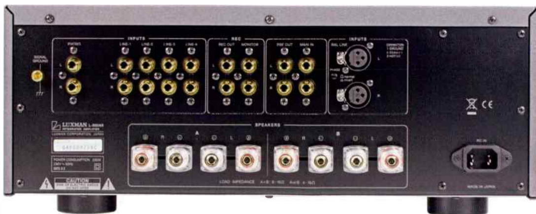
Connections include both balanced and unbalanced, as well as a phono stage in, pre-out and two pairs of loudspeaker terminals, A & B, that can be switched at the front panel, or turned off completely for headphone use.
