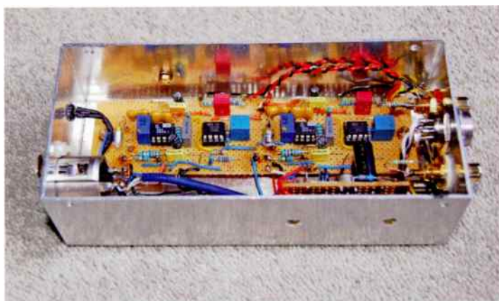
Fig 16 - The phono pre-amp. You can see four black silicon chips, two per channel, sitting in sockets.
