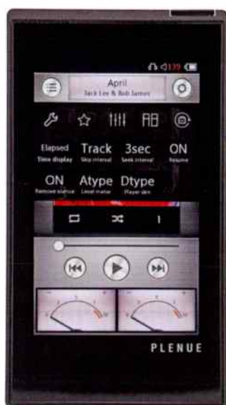
Yes – you even get output level meters on the Plenuie !! They are a display option, with red bar graph meters an alternative. Note the small red volume level readout at top right, and low resolution battery indicator – both difficult to read.
