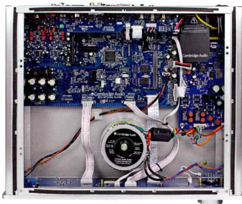
Inside, the Cambridge 851N uses a beefy toroidal transformer in its power supply. And just look at all those heavyweight digital chips...
