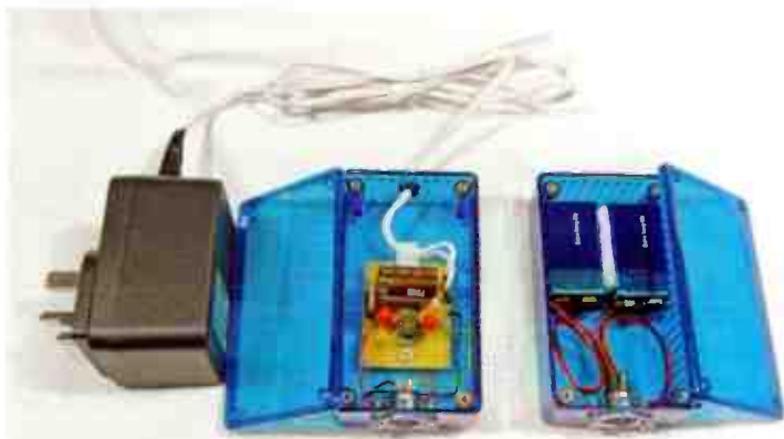
Fig 14. The power supplies: mains supply from a 24V a.c. wall wart at left, battery supply at right.
