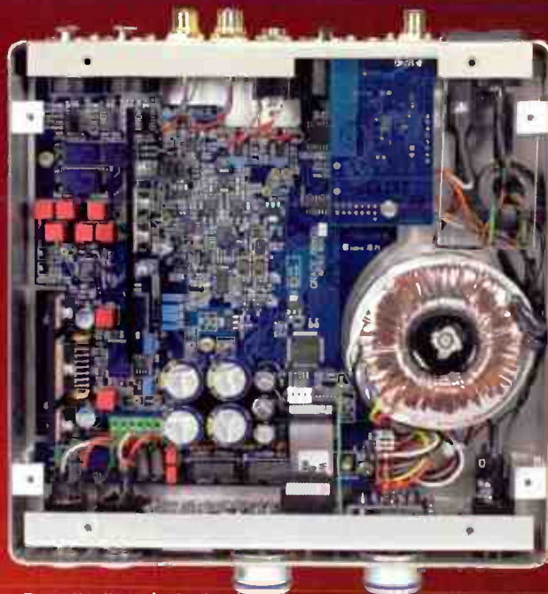
Despite its relatively small form factor the Grace uses a beefy toroidal transformer as the basis of its power supply.
