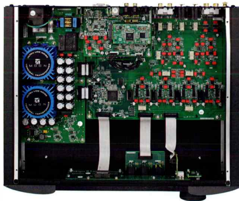
Twin toroidal transformers give the Moon Neo power to drive even the most insensitive of headphones.
