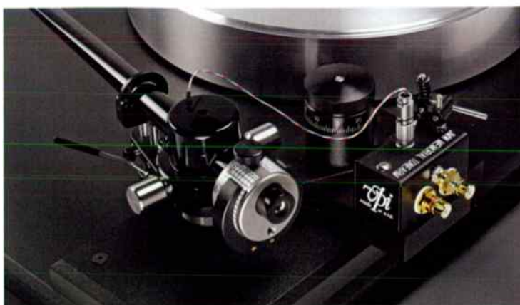
The VPI arm counterweight has a sliding sub-weight for fine adjustment, and is rotated for azimuth alignment. The lead-out wire unplugs, allowing the arm to lift-off for cartridge fitment.
