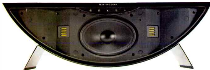
Behind the grille a central bass/mid unit is flanked by two of Martin Logan's proprietary Folded Motion tweeters - angled outwards to aid stereo dispersion.
