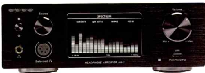
A bar graph display with short-term peak hold (red) reveals music energy spectrum.
