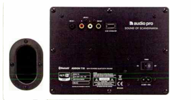
The rear panel includes a pair of stereo RCA line-level inputs, a 3.5mm mini-jack as well as a dedicated subwoofer output and a USB socket for charging portable devices.
