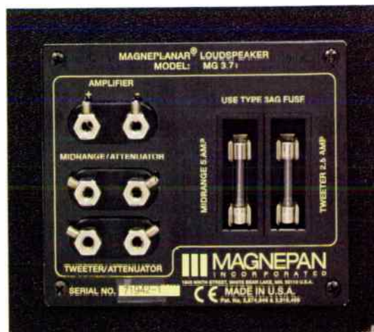
Rear panel of the main speaker. Note the ability to slot in resistors to attenuate the different panels to alter the frequency balance of the sound.
