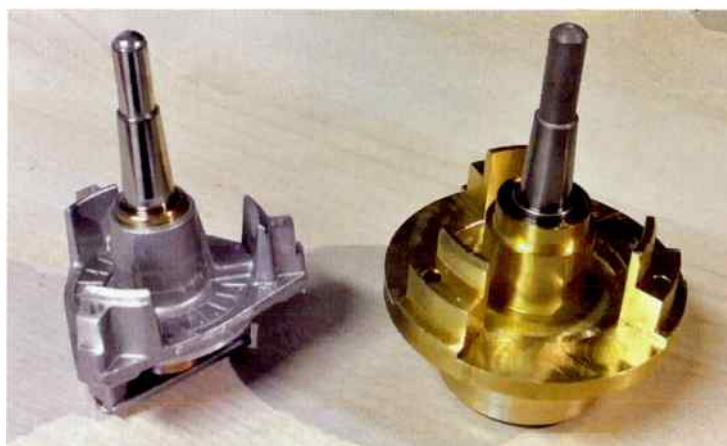
The Mike New bearing at right increased flutter at 6.6Hz from Technics 12 pole Direct Drive motor.
