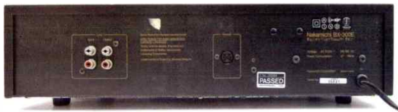
A simple rear panel carried audio inputs and outputs through phono sockets. No digital connectors here!
