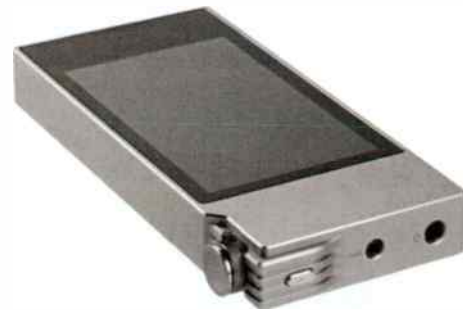
On top are a conventional 3.5mm headphone socket (at right), and rare 2.5mm four pole socket giving balanced output. Also, rotary volume control.
