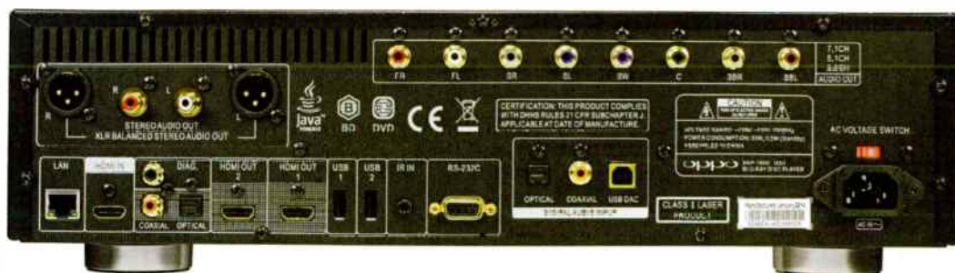
That this is a high resolution audio player is underlined by its balanced XLR outputs on the rear panel. There are two memory stick USB mass storage sockets, one HDMI input and two HDMI outputs, one streaming native DSD. Note also eight multi-channel audio outputs.
