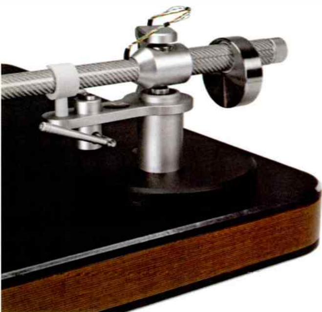
The arm is supported by magnetic bearings. Tracking force is adjusted by rotating the knob at the back of the arm. The arm height can be adjusted by slackening the hex nut, accessed through the hole on the mounting plate, and raising or lowering the arm by hand.
