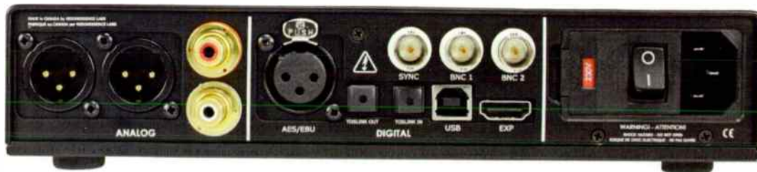
Comprehensive digital inputs and outputs include HDMI for video connection to a monitor.
