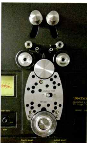
Tape transport. The direct drive capstan mechanism is based on the quartz-controlled, phase-locked servo system originally developed for the SP-10 Mk.II turntable
