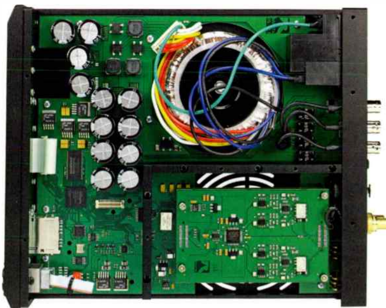
Inside, the Invicta Mirus features a sturdy line power supply, as well as two Sabre ESS DACs to give a class-leading 131db EIAJ dynamic range figure, our measurements show.
