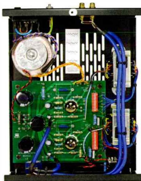
The dip switches to the right of the two ECL83 valves allow the user to set the impedance to match the headphones in use.
