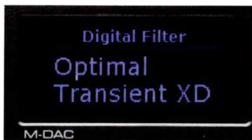
Digital filter selection is displayed on front panel. This is a 'slow' filter that gives best impulse response.
