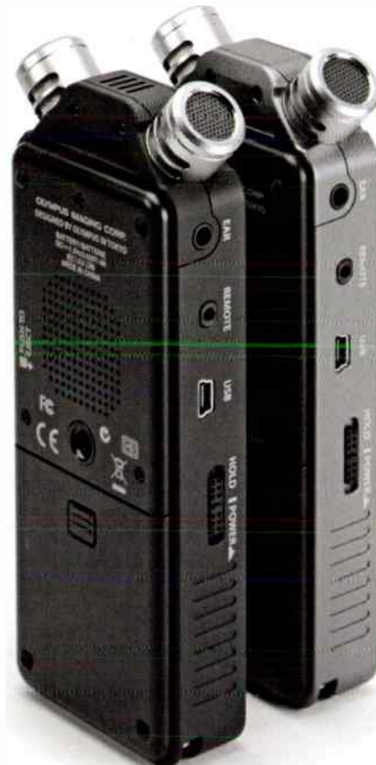
Small loudspeaker at rear, 3.5mm earphone and headphone jacks and mini-USB socket.
