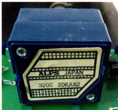
Money's put into where it counts – not silly gimmicks. The ALPS potentiometer seen here, used as a volume control, is the sort of component that you'll find in much more expensive gear.
