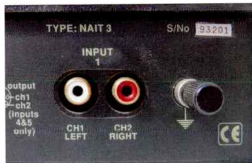
Although the other inputs used Naim's favourite locking-DIN connectors, the first input took the form of standard gold-plated phono sockets feeding a phono stage – note the ground post. It accepted line-level signals if the phono stage wasn't fitted.
