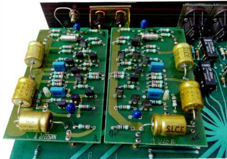
The NAIT 1 and 2 both had integrated preamps for MM cartridges. Owners of the NAIT 3 could, however, opt for an excellent internally-fitting phono stage. Versions that catered for MM (as seen here) and MC carts were available.
