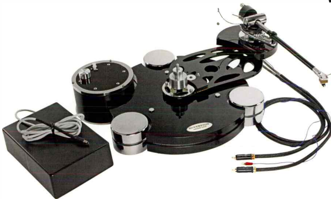
The 12in arm sits on an extended support. The motor sits in a cut-out and is moved to set belt tension. The arm cable is secured by a P clip in final assembly.
