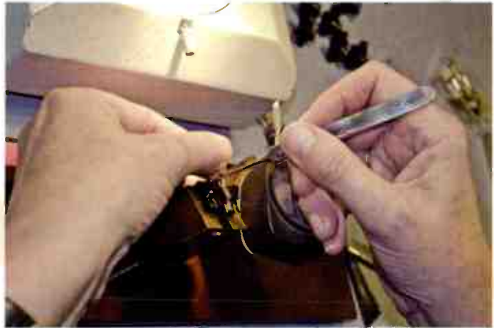
The completed assembly being inserted into the body. The rubber suspension is just being attached.
