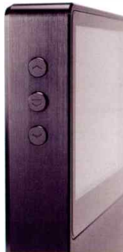
Small mechanical operating buttons offer track skip, play/pause.
