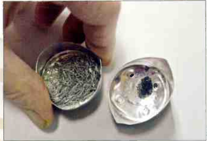
On the left are cantilevers; the 'dust' on the right is a large number of spherical styli.
