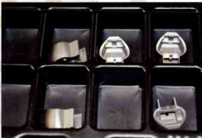
Here are titanium bodies for the Ortofon Anna cartridge. They are made by spraying 28 micron thick layers of powdered titanium, which is then melted by a laser to form the body.
