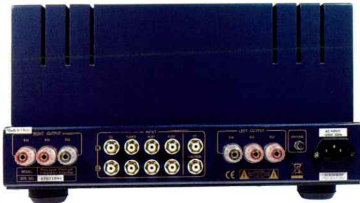
Four line level inputs, plus 4 Ohm and 8 Ohm loudspeaker outlets, on the rear panel.
