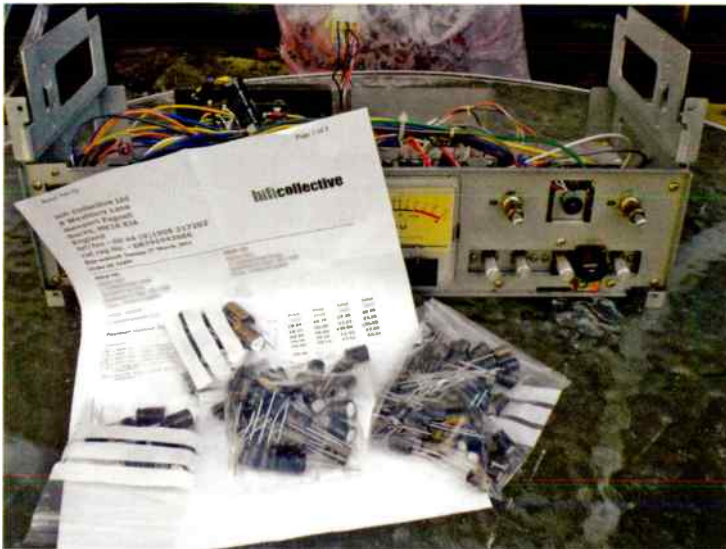
The circuits of tape decks, like most other audio equipment, contain a considerable number of electrolytic capacitors. Unfortunately, they eventually dry out and lose their effectiveness. These packs of replacement capacitors give you some idea of how many are fitted to the GX-630DB!
