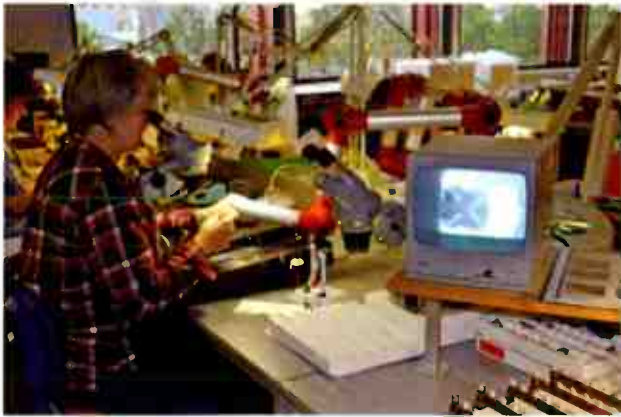
The coils are wound by hand, as seen in the screen on the right.
