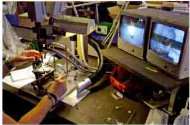
The stylus being attached to the cantilever. Two screens are used to ensure that the stylus is correctly aligned on the cantilever.
