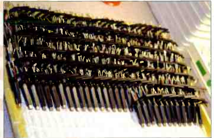
Completed Concord DJ cartridge bodies, awaiting fitment of the stylus assemblies.
