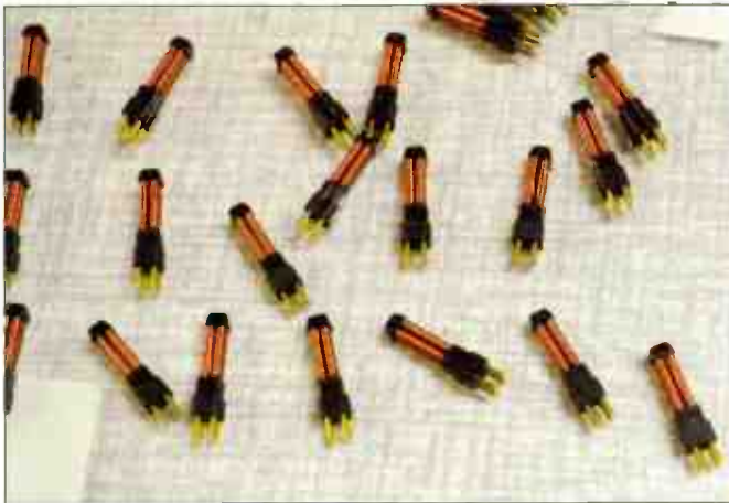
The coils are inserted onto Mu Metal pins. These pins are solid in the OM and DJ series of cartridges, while hollow ones are fitted to the 2M series.
