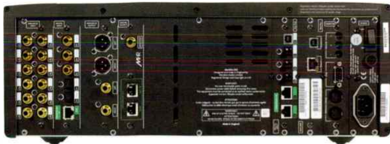
The 818 has a vertical array of unbalanced analogue inputs (left) via phono sockets. There are optical and electrical S/PDIFs too. Unbalanced and balanced (XLR) analogue outputs are fitted and these can feed any power amplifier.
