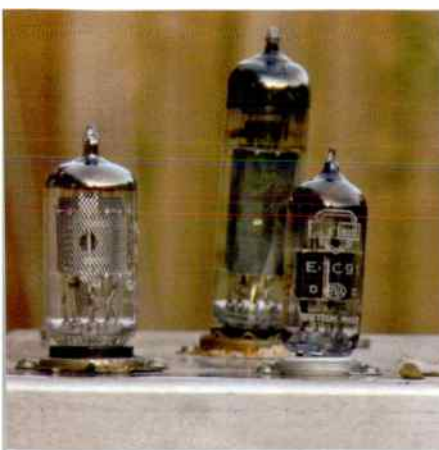
Unusual valve complement of an ECC91 as frequency splitter, anode driving HF and cathode LF crossover components, before triode connected EL84 in background. The EF86 provided voltage gain.
