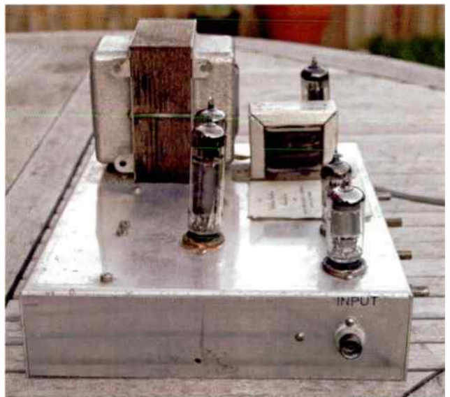
Single input on side of chassis, and note; with Haden's preferred RF / TV connector, rather than a nasty phono socket!
