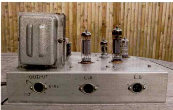
Rear view, and unusual use of DIN connectors; three pin type for both loudspeakers (no indication of which channel is doing what!) The six pin DIN carries Aux HT & LT supplies - dangerous!
