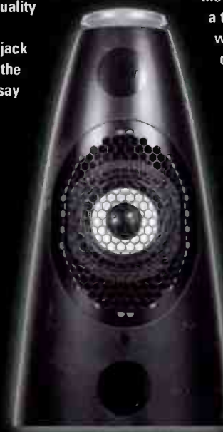
Meridian M6 loudspeaker 'all natural' – sack removed. At top is a single 3in full-range drive unit. Firing downward is a 6in bass unit, in a ported chamber. Inside each diagonally-connected M6 is a DAC, DSP processing unit TCVV power amplifiers.
