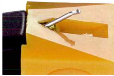
The tubular aluminium cantilever and diamond stylus of the MP-110. The MP-200 uses a boron rod as a cantilever.
