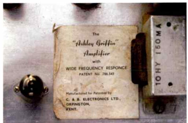
Proudly made by C&B Electronics, with Mr Griffin's patent number. Note the large choke, with no feedback around output stage. This was probably a necessity.
