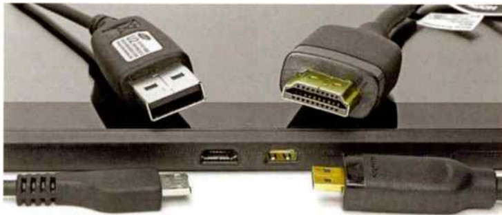
Micro USB socket at left and Micro HDMI multimedia socket at right, together with leads (not supplied).
