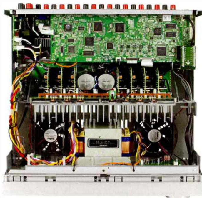
Two cooling fans cool the vertical heatsinks. Attached to them are seven amplifier boards in a row across the centre. The green board carries digital processing chips.
