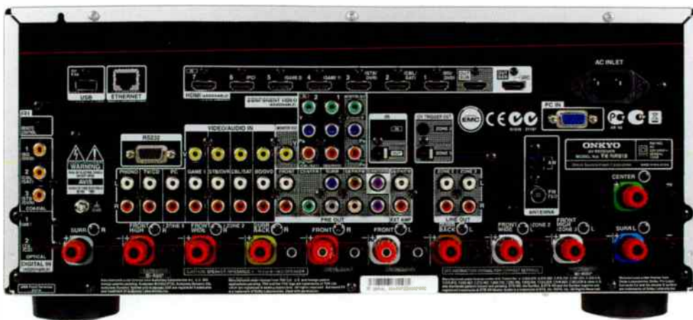
Digital inputs: USB, ethernet, and a row of HDMIs at top. There are also S/PDIF inputs – optical and electrical – at left. Seven amplifiers drive a 7.1 loudspeaker layout.
