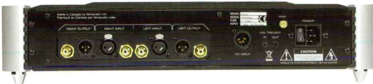
Unbalanced (gold) phono sockets and balanced XLR connectors on the rear panel, for both inputs and outputs. The XLR inputs have shorting links when not used, as shown.
