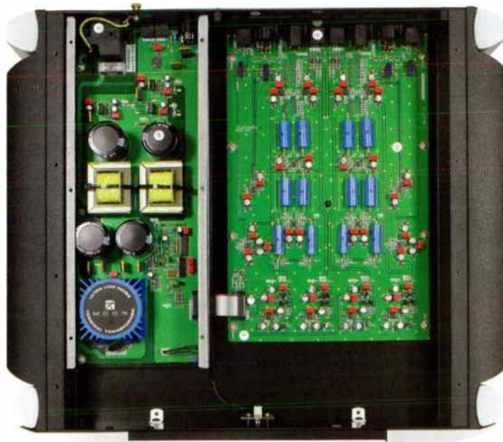
At left is the power supply complete with chokes, at right a multi-layer board, vibration damped, and carrying silicon chips.
