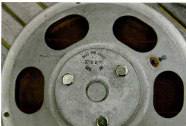
Rear of Philips 9710 'M' with pressed steel chassis and solid pole plates.
