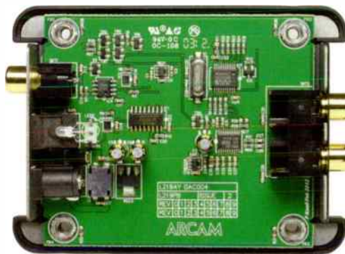
Miniature surface mount components and Burr-Brown PCM5102 DAC.
