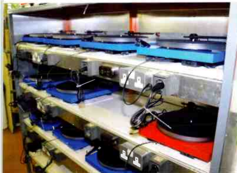
After assembly and calibration each turntable is then plugged in and left to run for 24 hours to ensure that it is working correctly. Note the variety of plug sockets for models for the UK, Europe and the USA.
