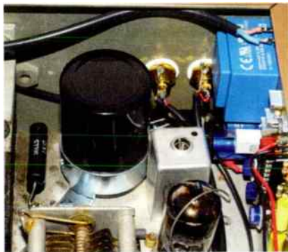
Mundorf HT capacitor and Mills series resistor fitted
