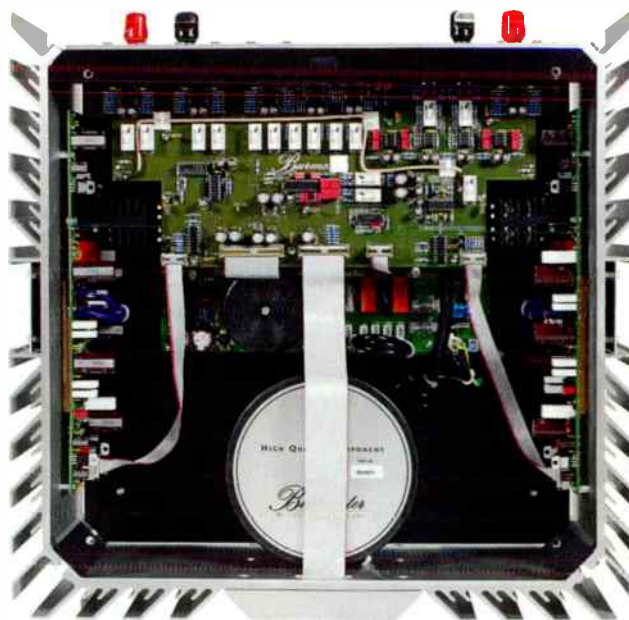
A big toroidal power transformer sits at the front of this amplifier, away from the signal input.
