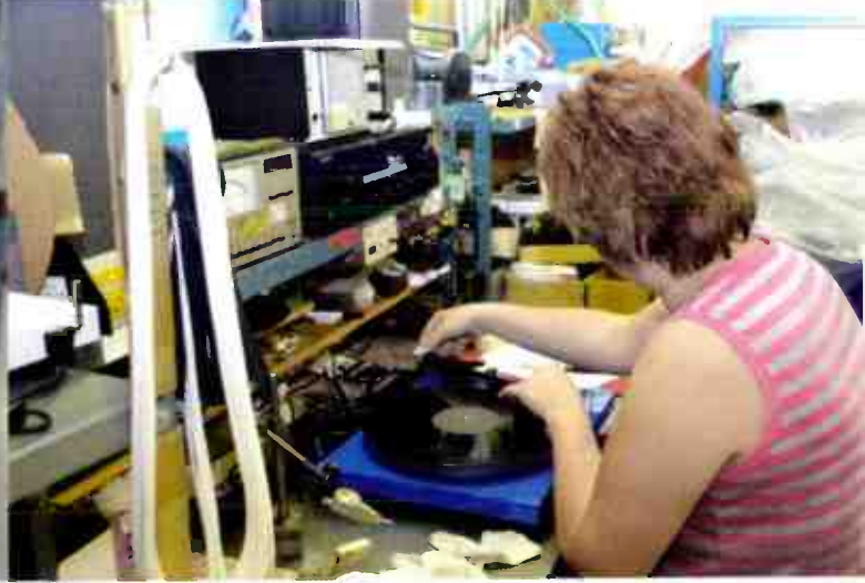
After assembly each turntable is calibrated and adjusted using a test record.
