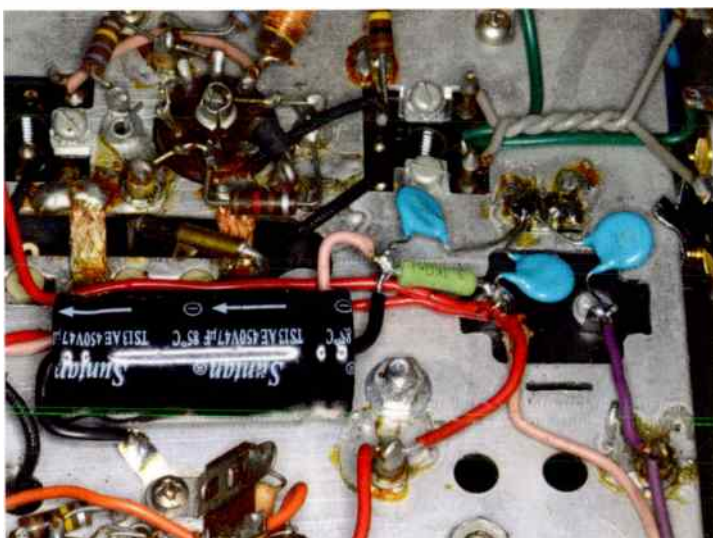
Chassis underside showing 3rd HT & bypass capacitors fitted
