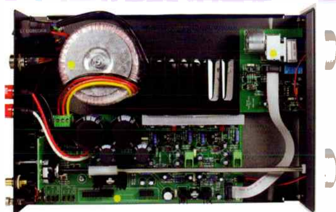
Heed Obelisk Si internal shows motor powered Alps volume control at (top right), and input selection with a rotary mechanical switch (bottom left).
