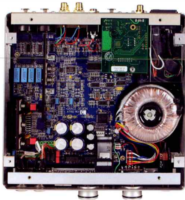
The internal circuit board is packed with miniature surface mount components. There are ten power supplies, a digital section, balanced input amps and display drivers. This is no simple headphone amplifier.
