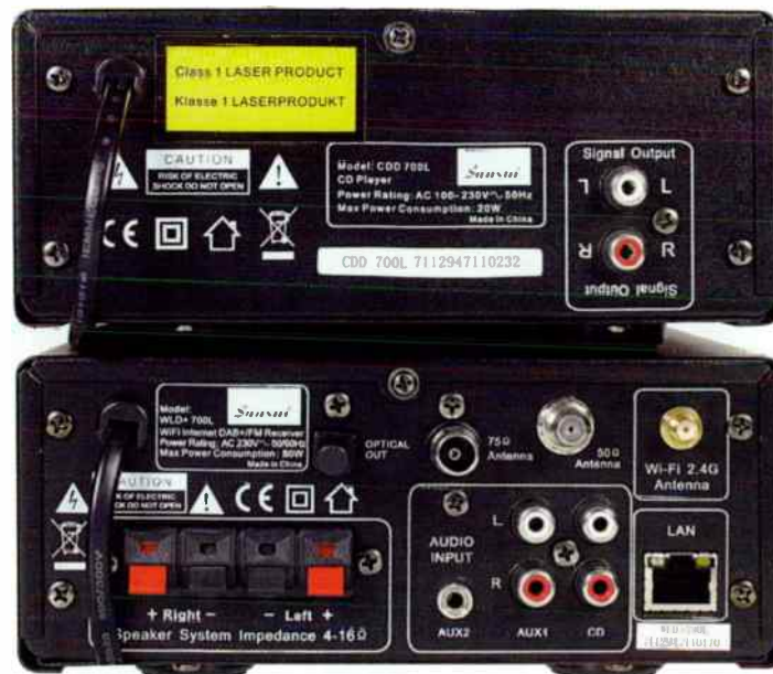
At top, CD player with one pair of analogue outputs. Below is the amplifier with a Wi-Fi antenna input, RJ45 ethernet socket, VHF aerial input, optical digital output, analogue inputs and spring clip 'speaker terminals.
