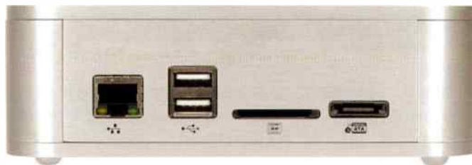
The left side panel carries an ethernet RJ45 socket, two USB 2 sockets, an SD card socket and an e-SATA input.
