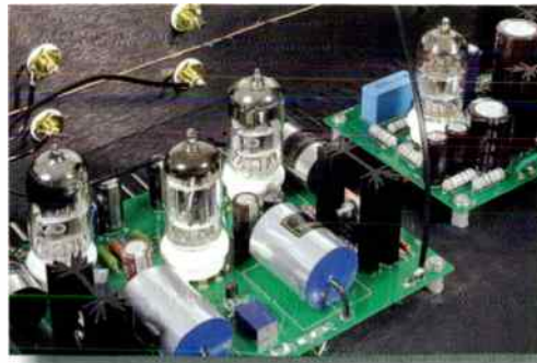
ECC88 low noise triode work with Toshiba JFETs in cascode arrangement. Output buffer/line driver is a 5687 double triode.
