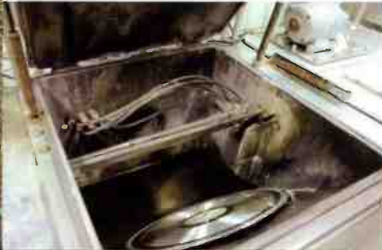
The lacquers undergo a silvering process. They spray two-to-three microns of silver over them.
