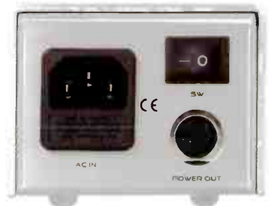
Rear of the power unit showing DIN power output and rocker style powerswitch.
