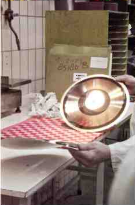
A stamper used to press the final vinyl.
