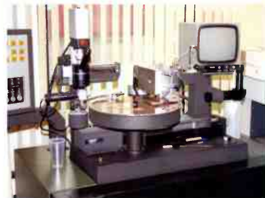
The DMM cutting machine in the mastering engineer's office.
