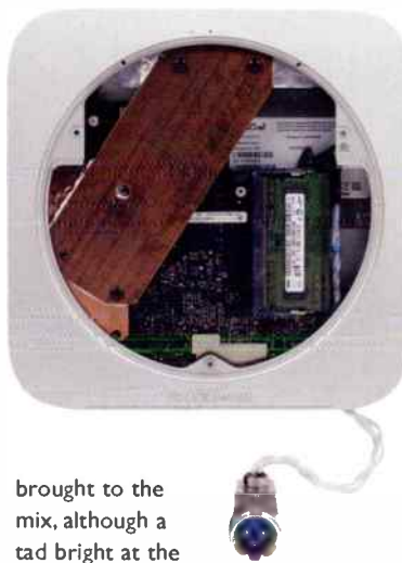
Inside a copper plate links the CPU to an aluminium block that replaces the old power supply.
