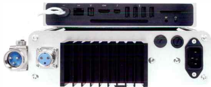
The modded Mini (top) has a power cord that plugs into the external Paul Hynes Bespoke supply.
