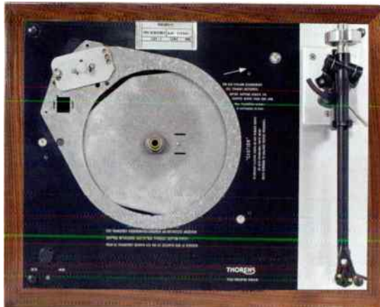
A new Origin Live d.c. motor, seen at top left of the platter, replaces the old a.c. synchronous motor. This makes speed control possible.
