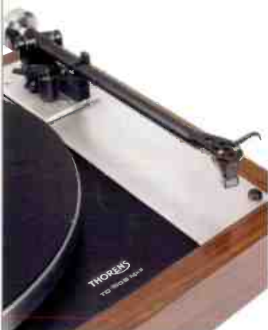
Rega RB251 arm with adjustable magnetic bias compensation and Ortofon Rondo Red cartridge.
