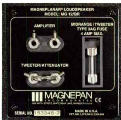
The small rear connection plate carries an unusual tweeter attenuator option.
