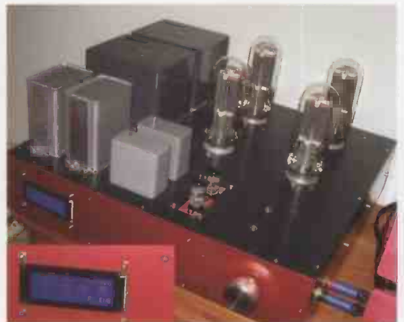
Mitch Long's impressive 211 valve amplifier - something to keep the air con. working in Singapore. Note the natty LCD display (inset) showing HT at 0.95kV. We hope the cat can read.
