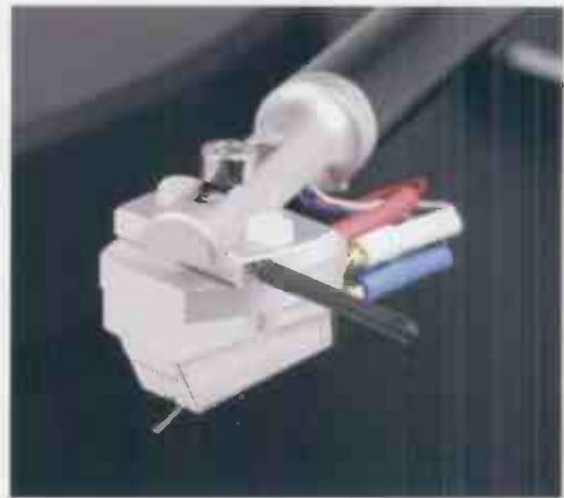
Headshell azimuth had to be adjusted by loosening a small lock screw.
