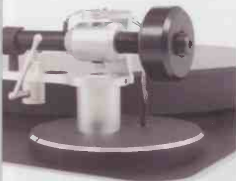
The Clearaudio Concept arm leadout wires are exposed.
