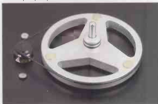
The drive belt can be left on the upper '33 1/3rpm' pulley when the external power supply is used.
