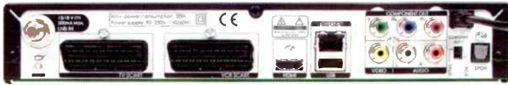
Rear panel of the Humax carries Scart, Component and Composite video outputs, plus analogue and digital audio outputs. The HDMI digital output carries HDTV.
