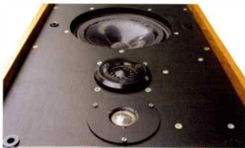
Spondor BC1 baffle showing Coles 4001G supertweeter.
