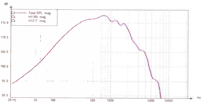
Fig. 1 - Effect of increasing bass unit series coil to 1.6mH to induce a falling upper midrange level
