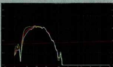
Green - Bass boost +6dB Red - Bass boost +3dB Blue - Bass boost 0dB
