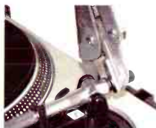
...and finally - time to remove the nasty stock Rega RB250 end stub, to fit the Michell TecnoWeight.
