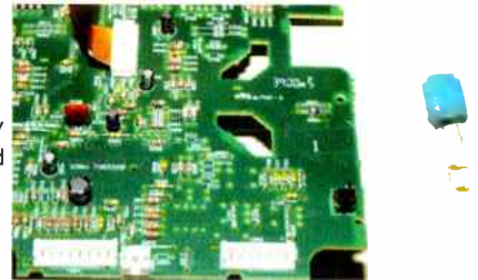
Drive crystal and capacitors removed.
