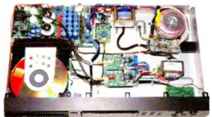
Completed upgrade with 3 clocks fitted.
