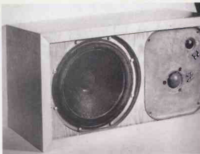
AR-3 prototype - an 'acoustic suspension' speaker that redefined loudspeaker design in the '50s.
