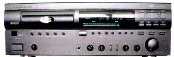
Philips Digital Compact Cassette was the first commercial use of 'Perceptual Coding', aka 'data reduction'...
