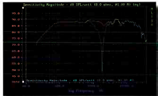
Graph 1. WD25T measured on treble axis at 1 metre. Blue trace shows effect of reversing phase to the treble unit.
