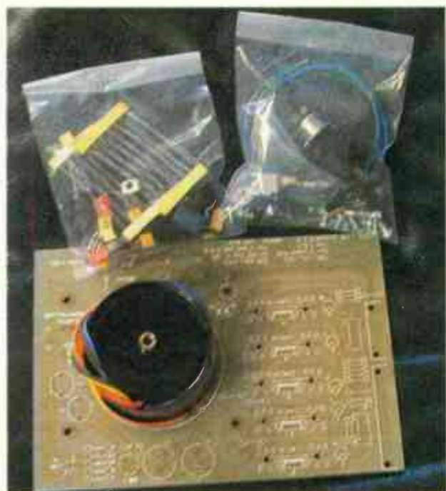
Power supply section as supplied.
