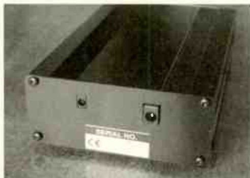
Figure 3. Rear view of the Ultra showing AC Input and DC Output Connections
