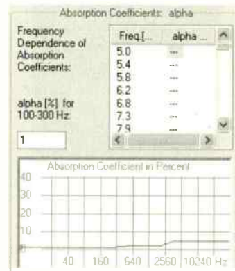
Cara room acoustics data for concrete, showing very low absorption.
