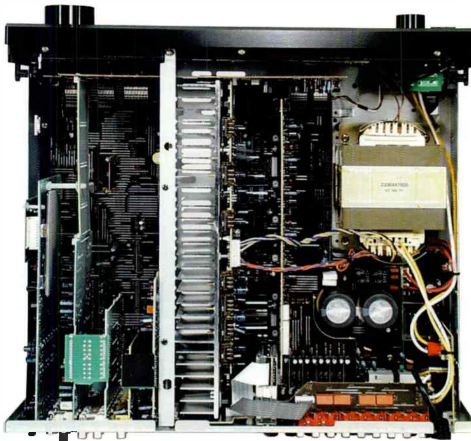
7 channels pushing out approximately 100 watts each makes for some serious heatsinking and a 'take no prisoners' power supply...
