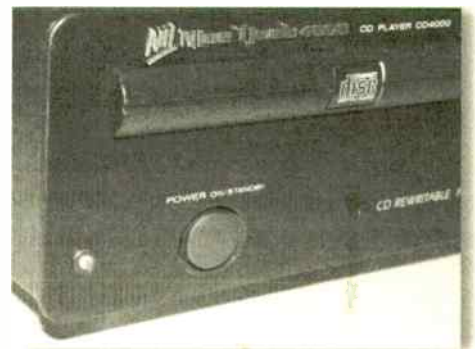
The additional power LED showing valve stand-by. Very few CD players have this!
