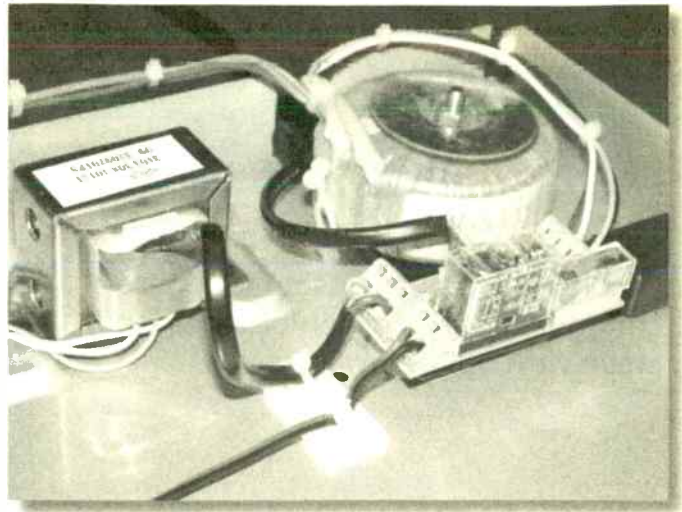
Mains transformers and power relay
