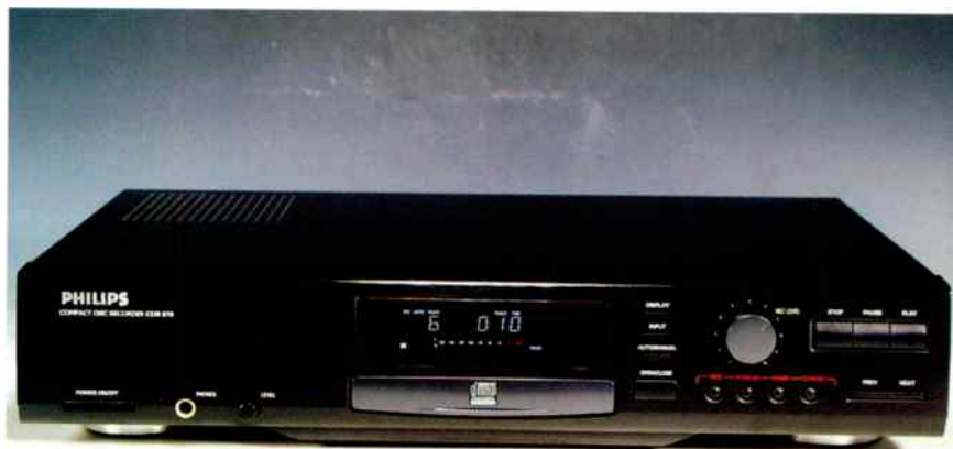
Philips' CDR 870 can record onto both CD-Recordable as well as CD-ReWritable discs.
