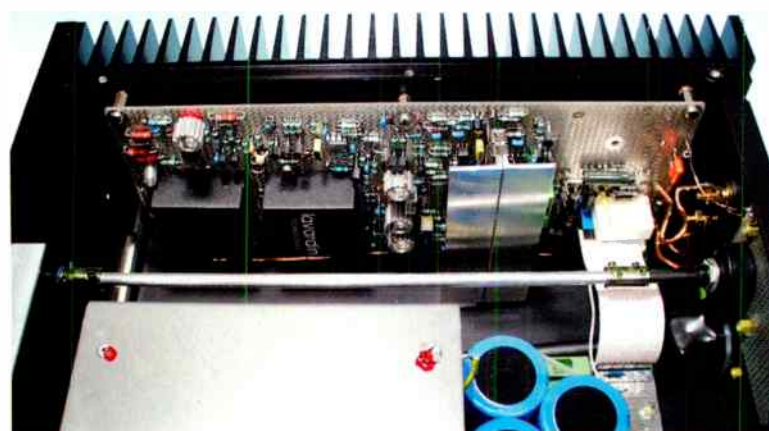
To the left of the PCB are the two black boxes which play a part in eliminating Memory Distortion. Shaft drive of the selector switch helps keep signal paths short.
