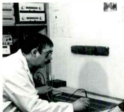
Checking the three bass stator sections to ensure continuity across them.
