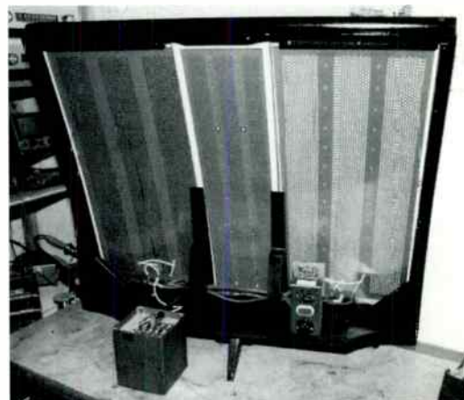
A rejuvenated '57, unclothed to show the central treble and two bass panels. The input transformer is sitting on the bench.
