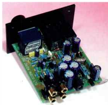
Inside the OBH-11SE, all circuitry is discrete.
