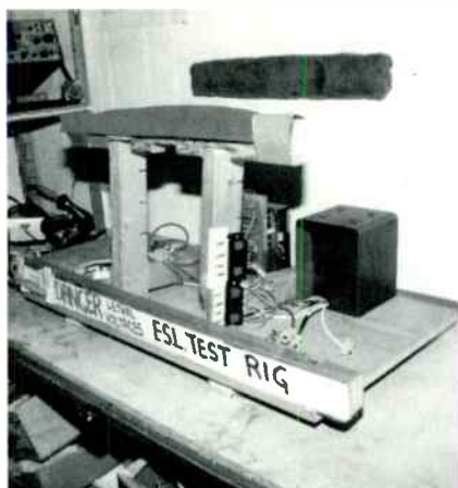
Soak testing of rebuilt panels is carried out on the test jig pictured above.
