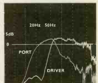
Fig 2 - This near-field response analysis of the PR240ZO bass driver and port clearly shows the operating range of each. As the port starts to resonate it acts against the driver, causing output to drop rapidly below 55Hz. Below this frequency the port radiates, extending bass response down to 20Hz.
