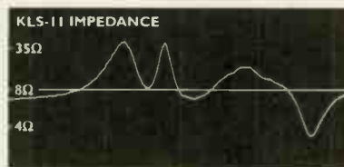
Fig 5 - Impedance was set to around 8ohms and measured out at 9.5ohms overall on a pink noise measurement signal.
