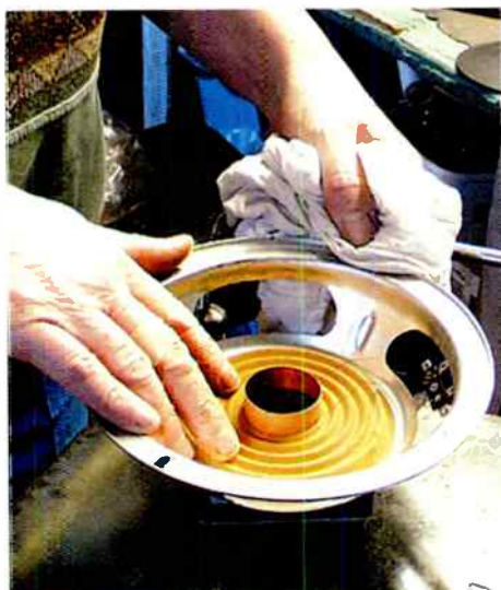
Fitting the voice coil and rear suspension.
