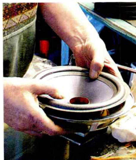
Aligning the new cone and surround.
