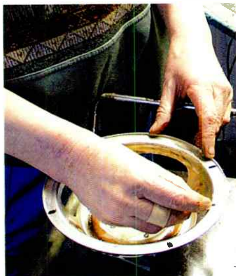
Removing the remains of the old surround.
