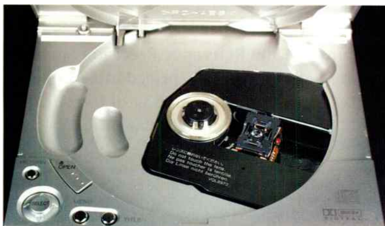
The spindle motor is a cut above the rest in terms of engineering. Here, it is allied to a robust dual-focus optical pick-up which slides along twin steel rails.
