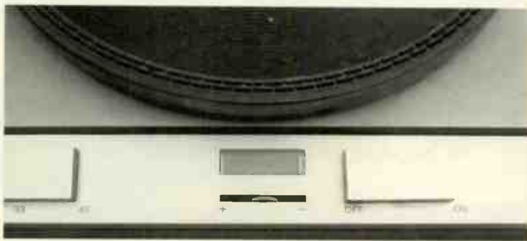
Thorens' TD125s rarely go wrong. The only area where faults tend to occur is in the pitch control slider.
