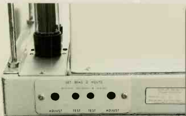
For the STA25 to work properly, the output valves need a bias of 2V, which is set with four potentiometers on the amp's back panel.
