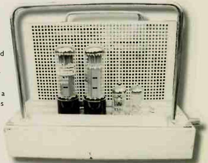
The STA25 uses a pair of relatively cheap, easily obtainable EL34 pentodes in its fixed bias output stage.
