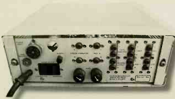
The CS22 pre-amp uses valves throughout apart from its phono stage which is a hybrid design that uses transistors alongside valves.
