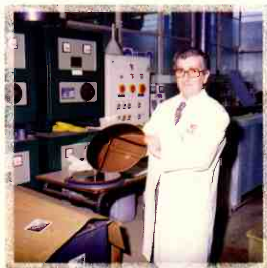
Bob Bailey in the plating shop with a Copper blank as used in Direct Metal Mastering.
