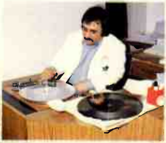
Quality control. A 'mother' is played by a Stanton 500AL cartridge in an SME3009 arm.
