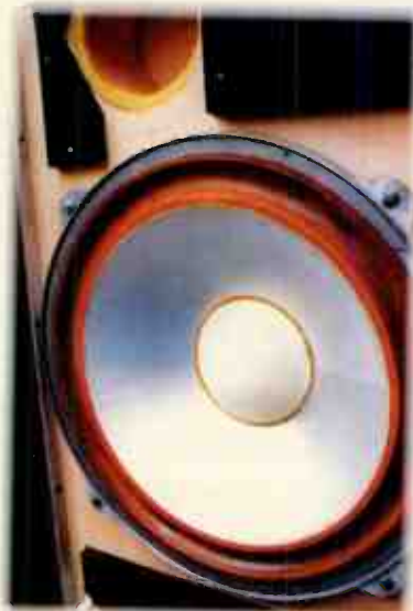
The Sandwich's cones are made of two thin sheets of aluminium glued to an expanded polystyrene inner.
