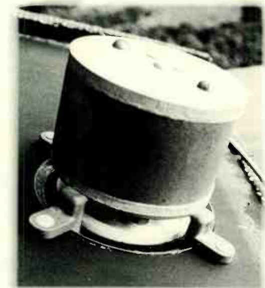
Both woofer and tweeter (shown here) use substantial high efficiency Alnico magnets.
