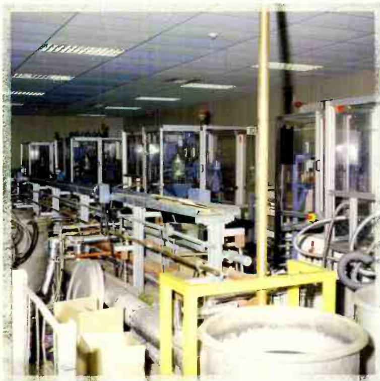
The main stamper shop. At right what looks like a vacuum sweeper hose sucks up vinyl pellets from a drum. The pellets are heated and compressed into a malleable ball ready for the press.
