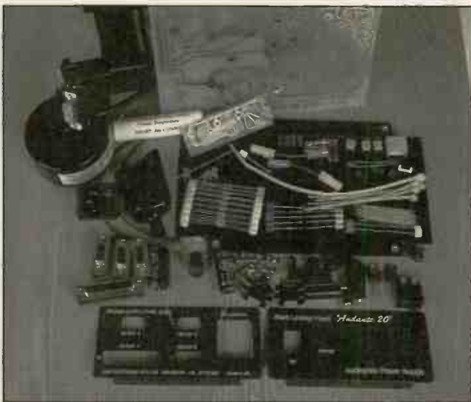
▲ The power supply module prior to assembly
