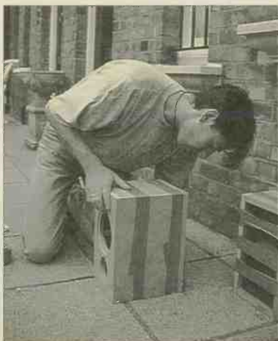
Use stretchy tape to pull the cabinet firmly into shape and leave to dry.
