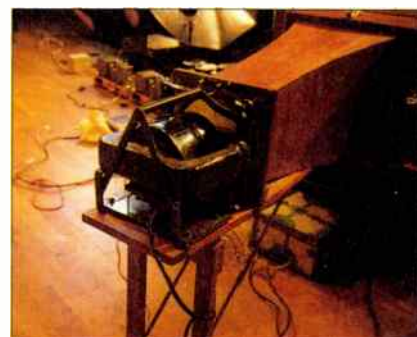
▶ ▶ Voigt's own twin diaphragm drive unit with sturdy forged iron frame.
