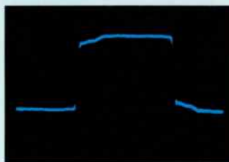
Absence of overshoot and ringing on a square wave shows that the Klyde cantilever is mechanically well damped.
