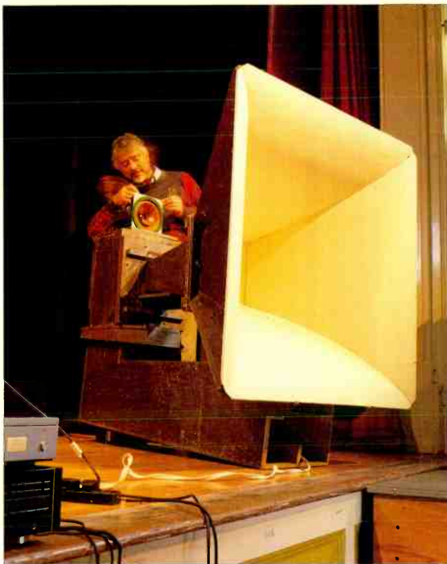
The newly discovered Tractrix horn being readied for use. It has a four foot square mouth and this version also has an additional forward firing bass tunnel slung underneath.
