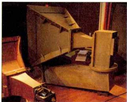
◀ ▶ Rear view of the horn, showing construction and the configuration of the bass tunnel.
