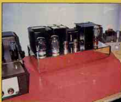
The home built Williamson design submitted by Alan Jones. In front are two KT66 output valves. Behind, its modern transformers are huge in comparison to those of the period, meeting Tim de Paravicini's interesting design criteria of "maximum iron, minimum copper" (see interview on p39).
