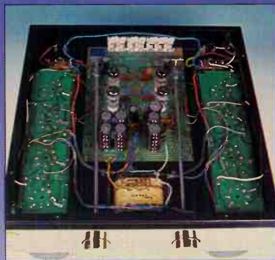
The preamplifier valves, which run cool, are hidden underneath. Long drive shafts to the rear mounted potentiometers keep leads short.
