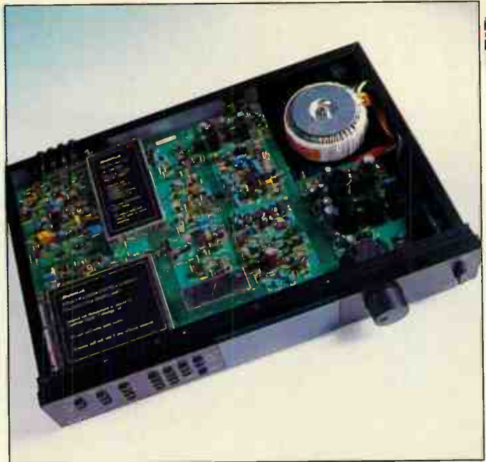
Audiolab's front end module and control microprocessor sit in metal screening containers to prevent interference.
