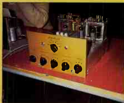
A rare 912 Plus from Denco of Claccon - the coil manufacturers. It was based on a GEC 12watt design. This one had Partridge transformers, adding to its value.
