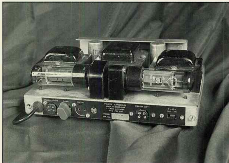
◀ The single-ended EL34 output valves were mounted horizontally to make the power amplifier chassis compact.
