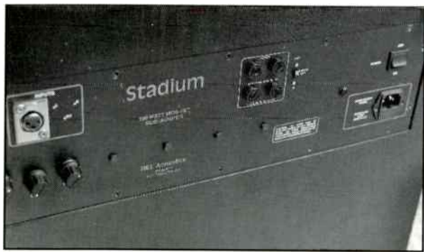
The rear panel has level and frequency adjustment controls at left, a Cannon input and amplifier protection fuses.
