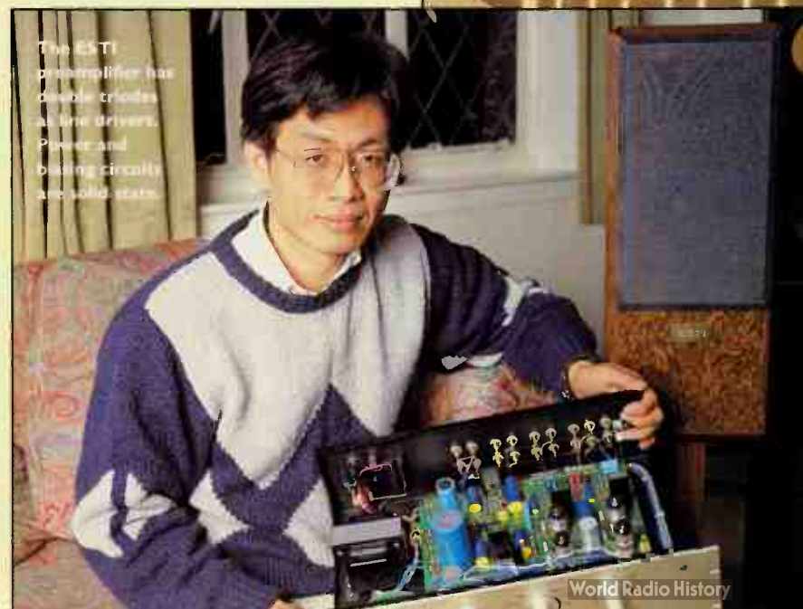
The ESTI integrated stereo valve amplifier uses two valves per channel, a double triode and a Western Electric 300B triode.
