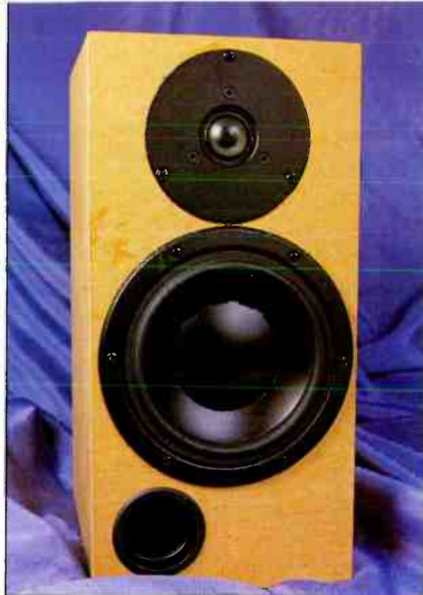
The finished loudspeaker in bare MDF, showing the quality of the drive units and the moulded plastic port that is provided.
