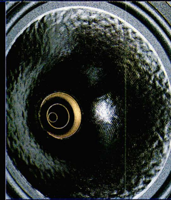
Top: the Kingdom's supertweeter and tweeter levels can be individually adjusted to taste. Above: the 12inch dual concentric with central tweeter. Below: note the earth post next to bi-wire speaker sockets.
