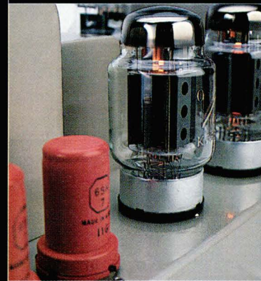
Above: the reborn Quad pre/power amp combo. Below, from top: The power amp's KT88 valves give it a healthy 40 Watt output; The QC-24's volume control is reminiscent of the original 22; Modern components help the new Quads shine.
