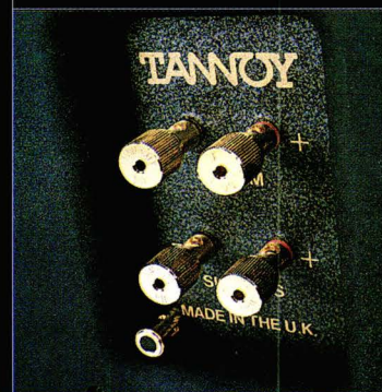
Top: the Kingdom's supertweeter and tweeter levels can be individually adjusted to taste. Above: the 12inch dual concentric with central tweeter. Below: note the earth post next to bi-wire speaker sockets.
