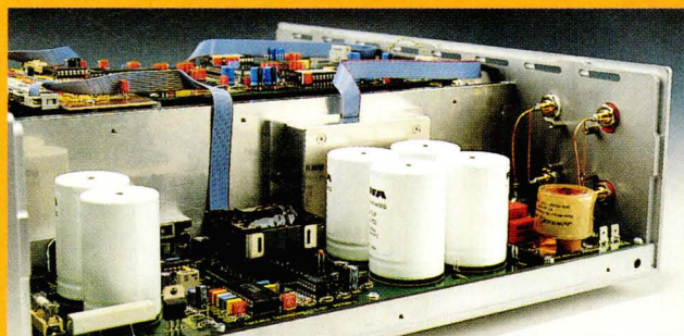
The 'brains' of the Millennium are on the circuit board shown top left in this photo. Pictured below right is an annotated plan view of this board. Beneath the PCB is a large toroidal transformer.
